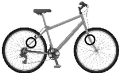
Loosen the screw on the clamp to open it. Position the clamp around the bike frame so that the clip mouth is facing the wheel spokes and tighten the screw.
